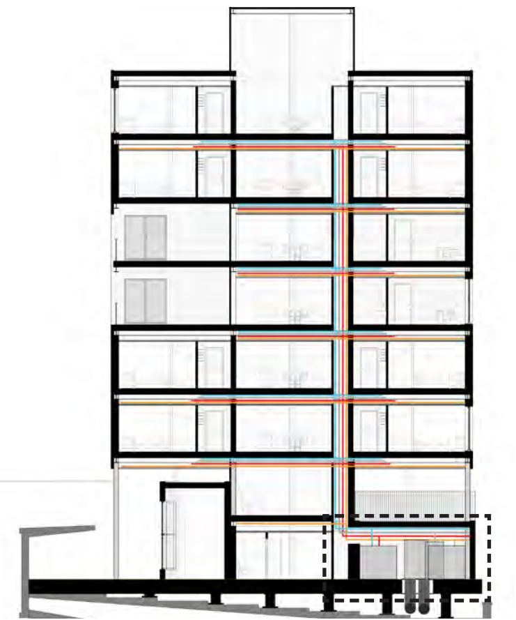
Diagrammatic building servicing strategy Ground floor plant room services are connected to main power and water supply through insulated duct pipes underneath the foundation slab to the main Tempelhof building.
